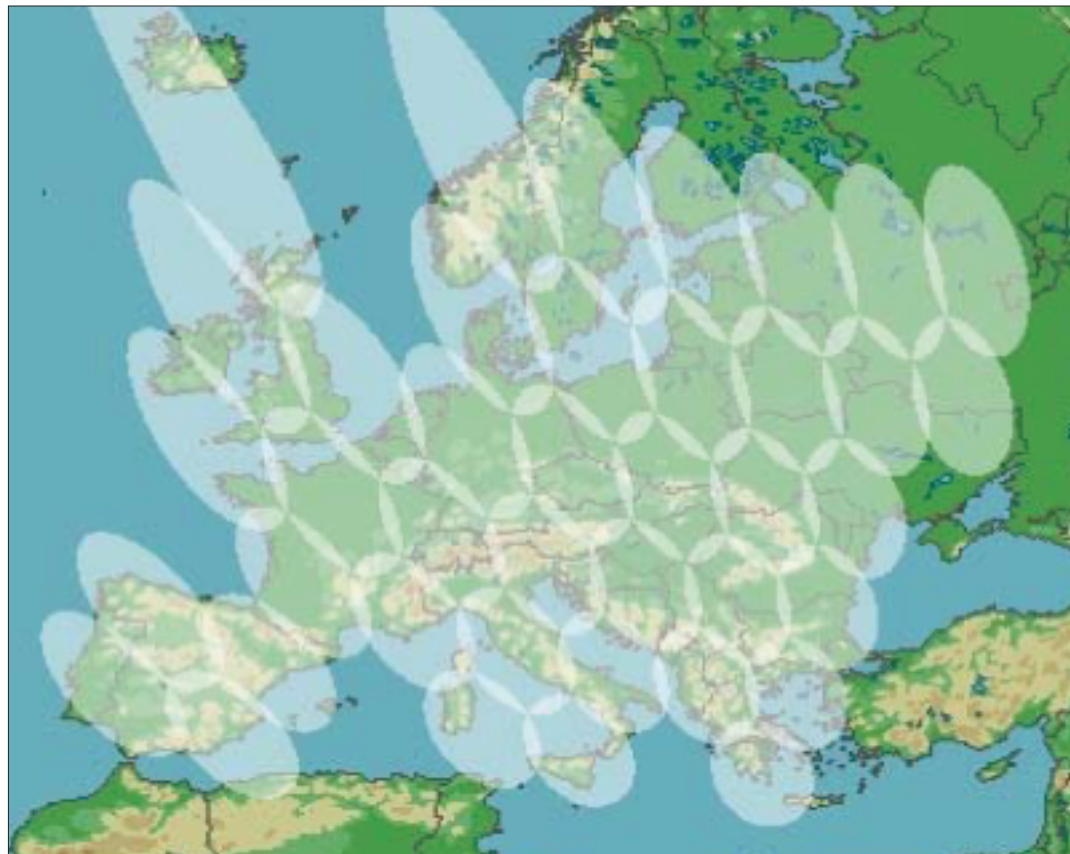
■ Figure 4. 40 Ka-band spot beams -3 dB contours over typical European coverage.
